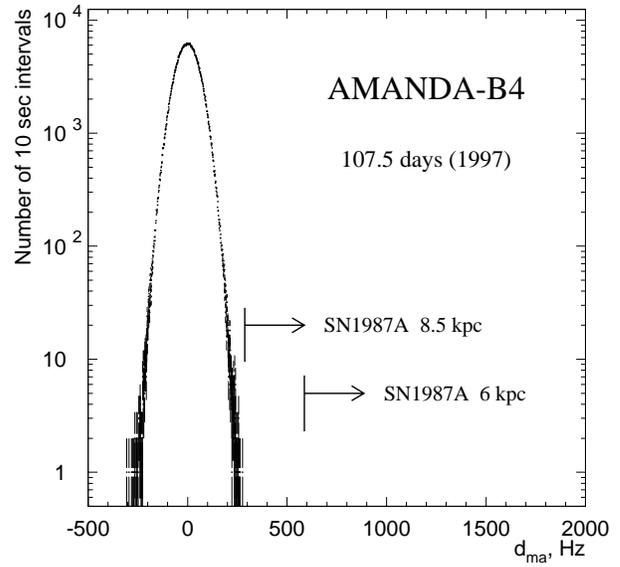
Figure 4: Deviation  $d_{ma}(t)$  of the summed noise rate from the moving average for the selected 51 PMTs of AMANDA-B4 and a selected life time of 107.5 days in 1997, with a cut in  $\chi^2/NDF \leq 1.5$ . Indicated are the cut-values for signals expected for SN1987A-type Supernova at 6 kpc and 8.5 kpc.
