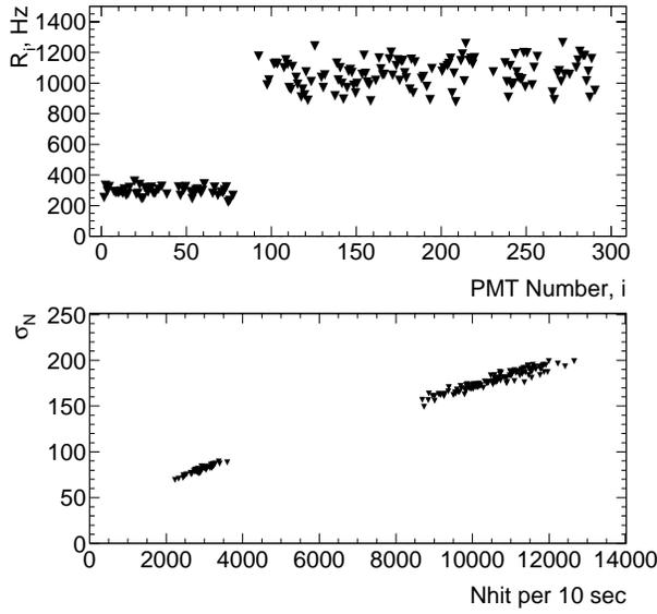
Figure 1: (Upper:) The average noise rate,  $R_i$ , for the selected PMTs; Strings 1-4:  $i = 1-80$ , strings 5-10:  $i = 87-302$ . (Lower:) Width of the noise hit distribution,  $\sigma_N$ , as function of the average number of hits  $N_{HIT}$  in 10 sec intervals.
