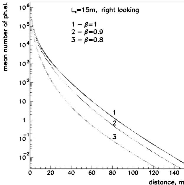
**Figure 1:** Expected numbers of p.e. versus distance from monopole track to OM
