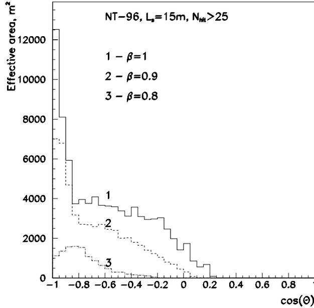
**Figure 2:** Effective area of *NT-96* for fast monopole detection in the first approach.
