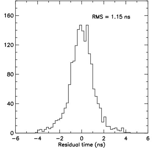
Figure 3: Timing residuals for one STACEE channel relative to the best fit spherical wavefront.
