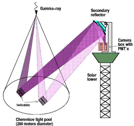
Figure 1: Concept of solar tower Cherenkov detection of gamma-ray air showers.
