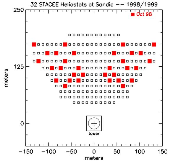
Figure 2: Plan view of NSTTF facility in Albuquerque, NM indicating 32 heliostats used for STACEE since October 1998. STACEE will expand to 64 heliostats in the year 2000.
