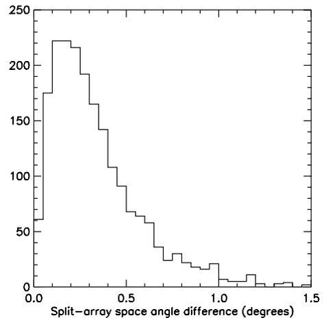
Figure 4: Distribution of space-angle differences between overlapping sub-arrays for cosmic rays detected by STACEE. The median difference of about  $0.2\text{--}0.3$  degrees provides an independent estimate of STACEE’s angular resolution.
