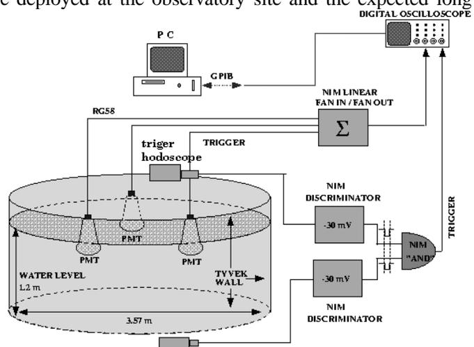
**Figure 1:** Schematical view of the WCD Prototype at Puebla operating to obtain VM.
