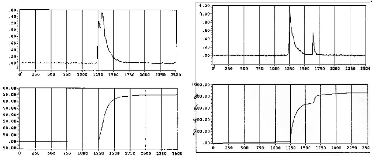
**Figure 3:** Two examples of recorded events with WCD structured signals. Left (right) picture shows signals with integral charge  $Q=84$  VEM (40 VEM),  $t_{50\%} = 27.47$  ns. (25.32 ns.) and  $t_{90\%} = 94.05ns.$ (161.41ns.)
