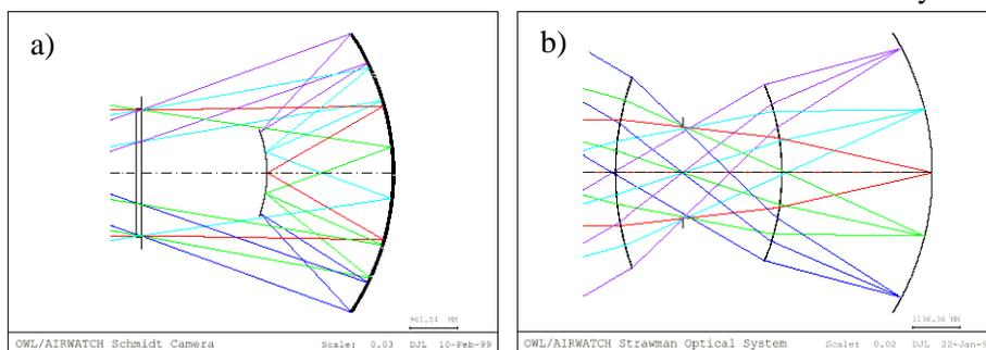
**Figure 3:** a) Optics using Schmidt lens configuration. b) Optics using double Fresnel lens configuration.
