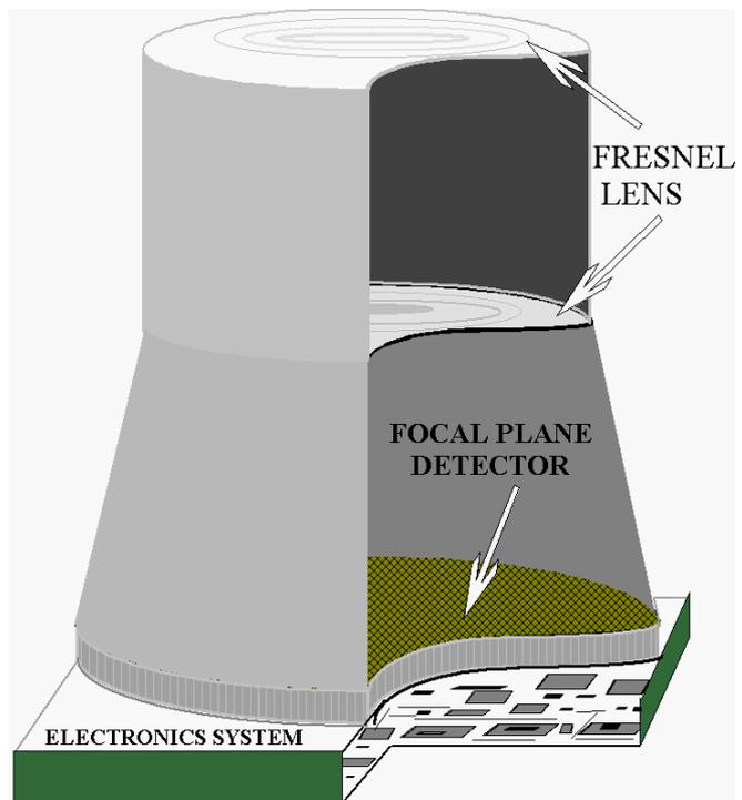
**Figure 2:** The OA instrument in its main parts. A configuration using Fresnel lens here
