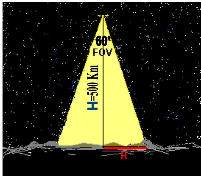
**Figure 1:** Important parameters that contribute to the huge geometrical factor of the OA experiment are: observation altitude and instrument FOV.
