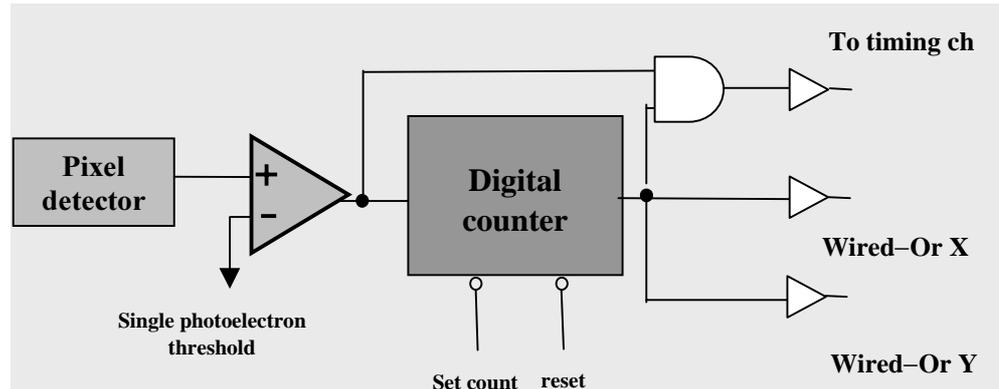
**Figure 5:** Block diagram of the pixel front-end electronics.
