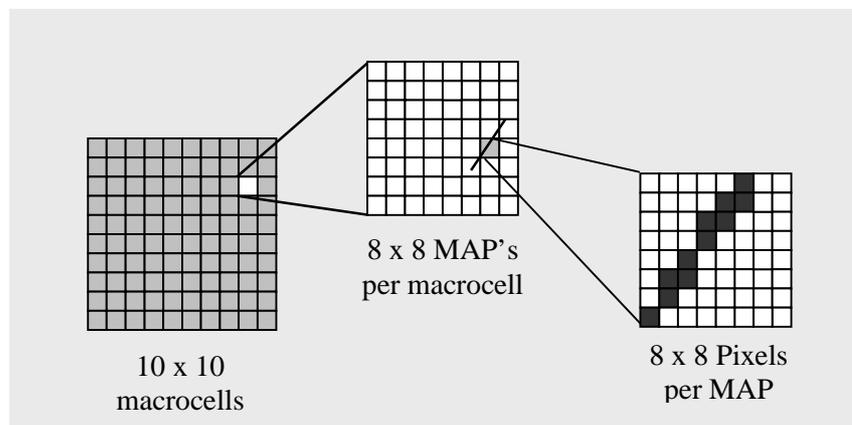
**Figure 4:** Schematic view of the modular focal plane. A Solution using 64 pixels Multi-Anode Photomultiplier R5900-64 (8 X 8 pixels) is shown. The focal plane macrocells are 100 with 64 MAP's per macrocell.
