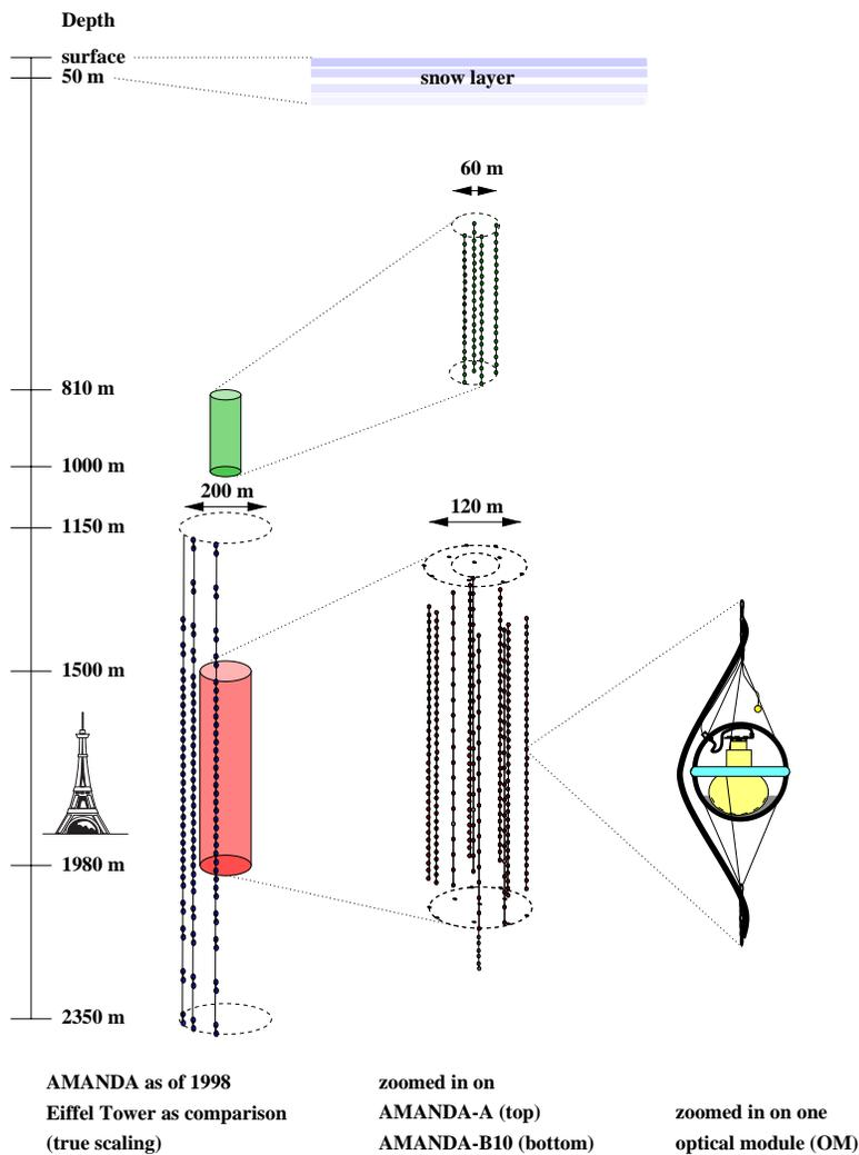
**Figure 1:** Schematic diagram of the AMANDA detectors.
