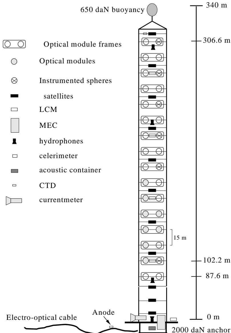
**Figure 2:** Schematic view of the prototype string.
