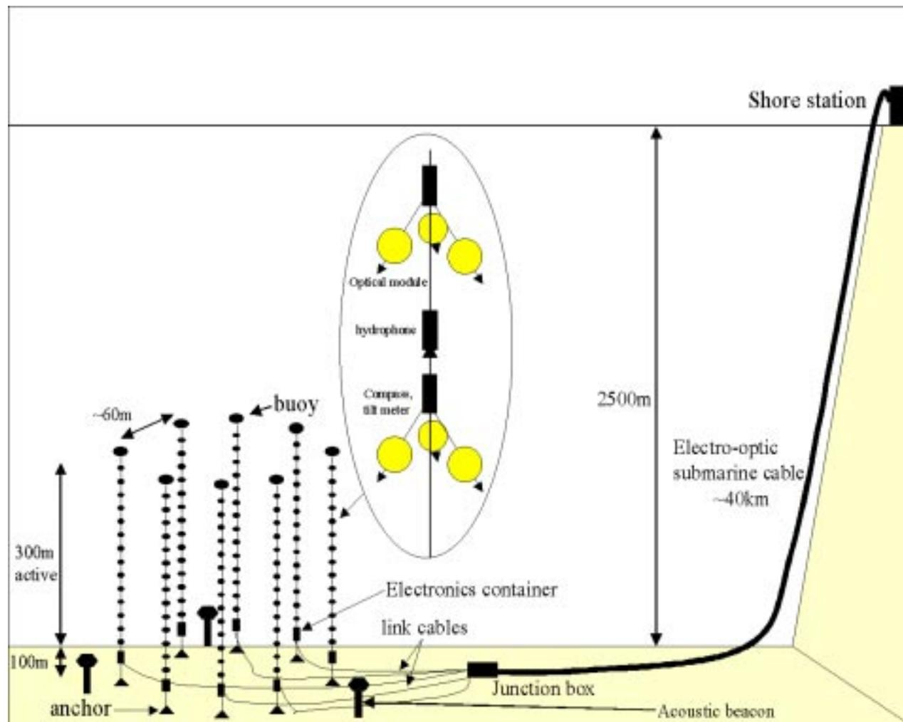
Figure 1: Schematic diagram of the first phase of the ANTARES detector.
