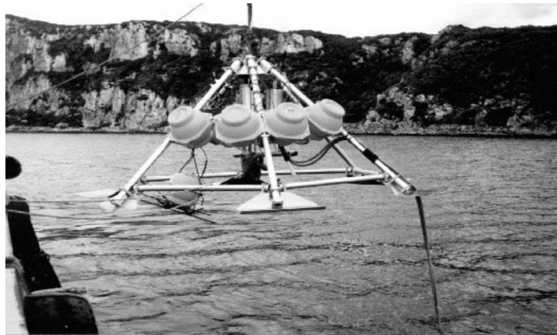
Figure 2: The Anchor + Environmental Unit during the deployment in the shallow water
