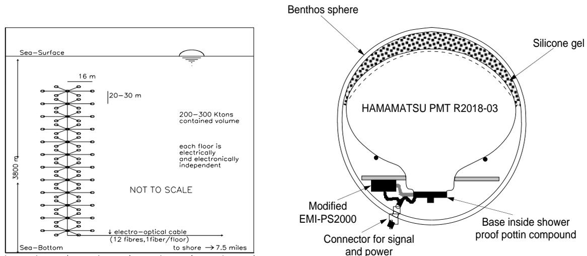
Figure 1: Schematic view of NESTOR tower and optical module
