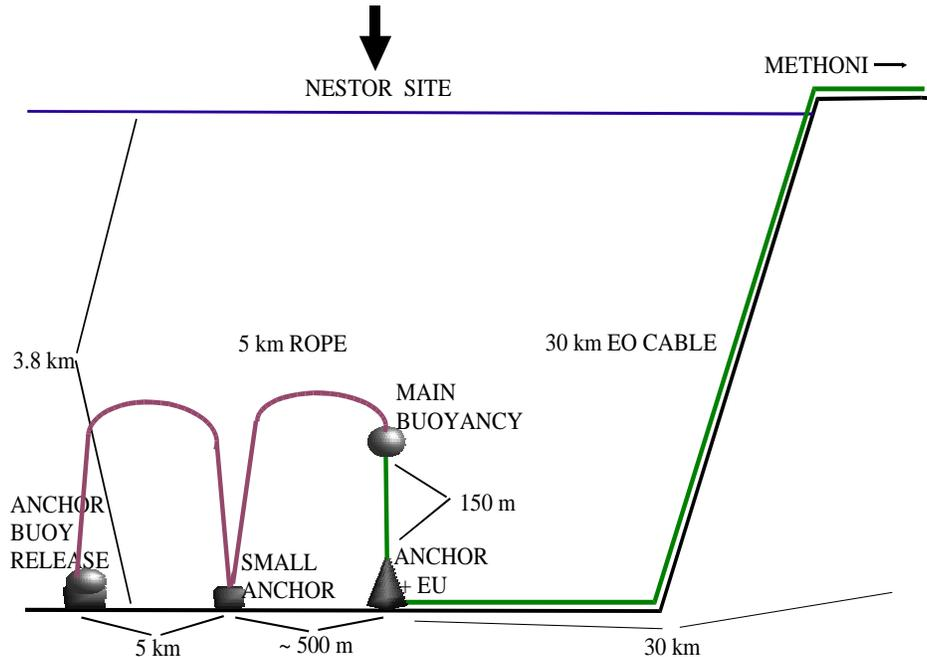
Figure 3: Schematic view of cable deployment
