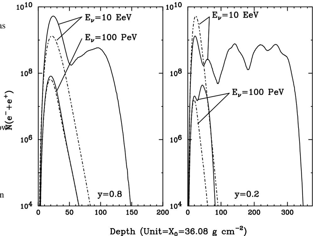
**Figure 1:** Longitudinal development of hadronic (dashed lines) and mixed showers (continuous lines) initiated by neutrino interactions in ice for different values of neutrino energies and  $y$ , as marked.
