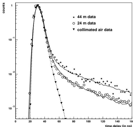
Figure 4: Distribution of photons arrival times for a collimated air spectrum (dashed curve) and for two spectra taken *in situ*, with source-deflector distances of 24 m and 44 m. All spectra are normalized to a maximum of 1. *In situ* spectra are corrected for the  $1/D^2$  decrease. Note the strong suppression of the scattering tail as compared to the direct peak. The Monte Carlo spectra for the best-fit values are overlaid (full curve) on top of the data.
