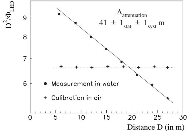
Figure 1: Effective attenuation length obtained with the DC measurements.  $D$  is the distance between the source and the phototube,  $\Phi_{LED}$  the LED luminosity required to obtain a constant current on the phototube.
