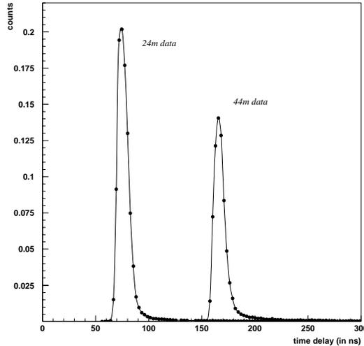
Figure 3: Distribution of photons arrival times for two source-deflector distances: 24 m and 44 m.
