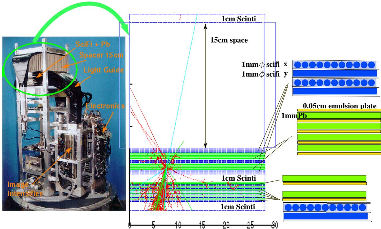
Figure 1: The BETS scintillating fiber imaging calorimeter. The vertical 1.5 cm thick scintillator plates are being implemented newly.
