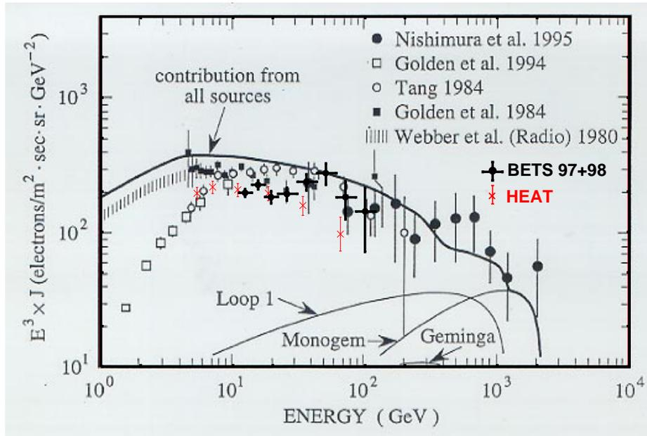
**Fig.3:** Comparison of our results (BETS 97+98) with the all-electron flux of HEAT and previous observations. Solid line presents the calculated spectrum by a diffusion model for all sources; dotted the nearby sources.
