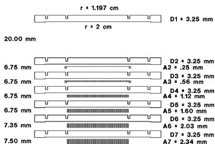
Figure 1a: Electron Telescope Schematic
