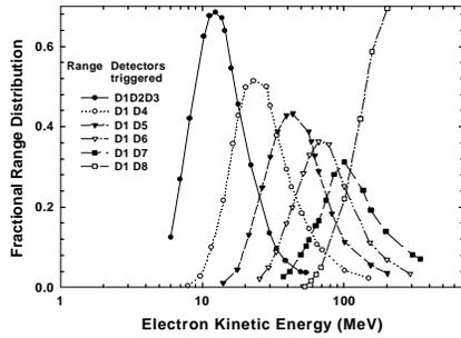
**Figure 1b: Electron-calibration results for prototype Voyager Electron Telescope. The response curves shown represent the fractional distribution of mono-energetic electrons over the telescope ranges.**
