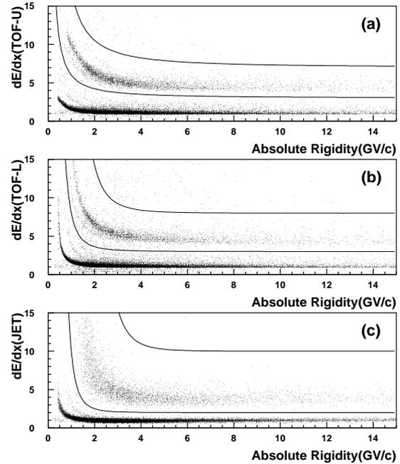
Figure 1: The  $dE/dx$  vs. absolute rigidity measured by (a) top and (b) bottom TOF and (c) JET. Because of the energy loss in the detector, the  $dE/dx$  in the bottom TOF is slightly higher in the low-rigidity region.
