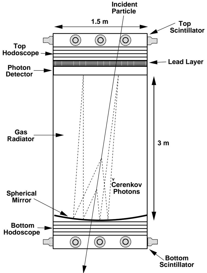
Figure 1: The RICH instrument in cross section
