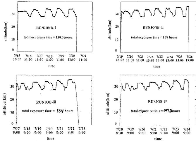
The trajectories of the balloons in 1995 and 1996 campaigns are shown in Fig.1. Trajectories in 1997 is not shown but very similar to those here. The trajectories are impressively stable. The altitude profile of the balloon flights are shown in Fig. . We can see the variation of altitude due to sun radiation.
