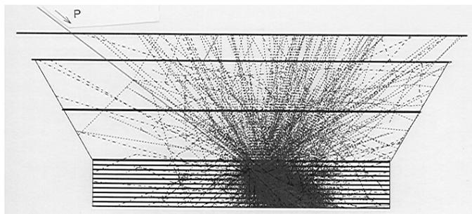
**Figure 2:** Simulated 1 TeV proton shower in the CREAM calorimeter.
