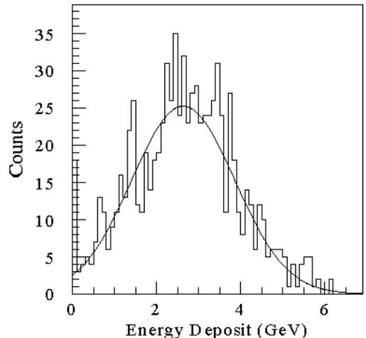
**Figure 3:** Simulated energy deposit in the W-Sci calorimeter for vertically incident 1 TeV protons.
