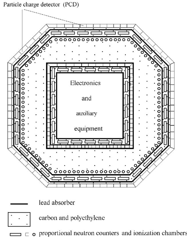
Figure 1: Cross section of the Ionization-Neutron CALorimeter (INCA) with the Particle Charge Detector (PCD). Basic parameters are: weight = 4.6 - 9 t;  $S\Omega = 10 - 30 \text{ m}^2\cdot\text{sr}$  (up to 20 - 60  $\text{m}^2\cdot\text{sr}$  for iron nuclei); height = 1.5 m; diameter = 1.8 - 2 m; absorbers are carbon and polyethylene.
