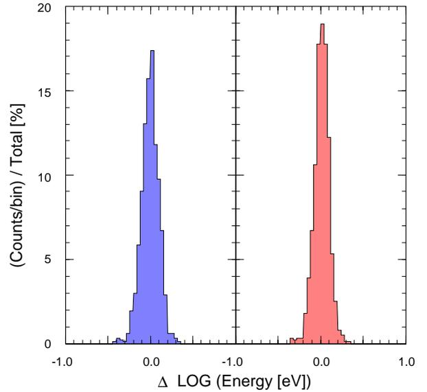
**Figure 1:** Accuracy of event reconstruction. Fluctuation of energy determination for  $3 \times 10^{19}$  eV (left) and  $10^{20}$  eV (right) showers with zenith angles less than  $45^\circ$ .
