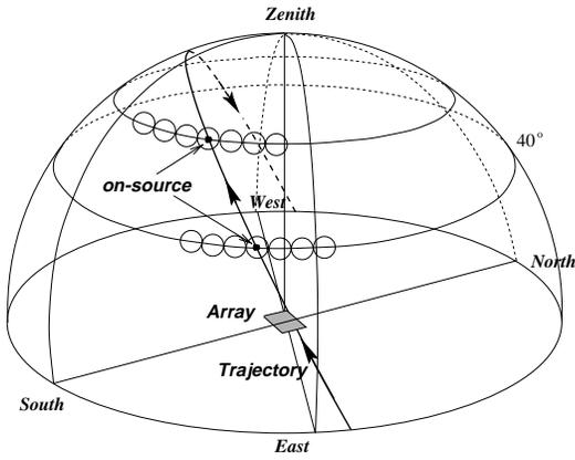
Fig. 2. Schematic view of the equi-zenithal scan method.
