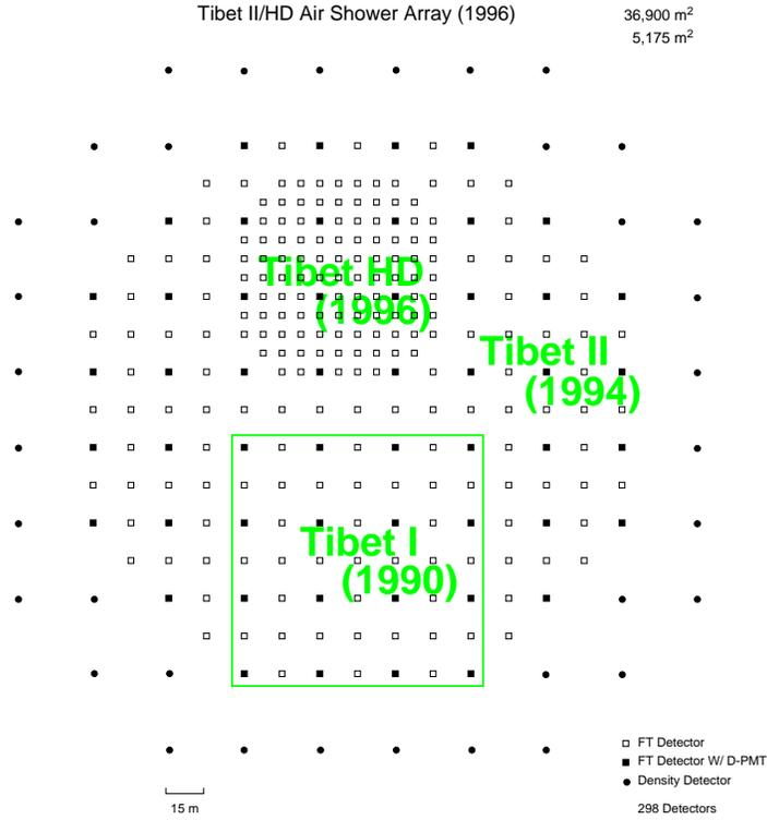
Fig. 1. Schematic view of the Tibet air shower array (Tibet I, II and HD array). Open and Closed squares are equipped with fast response phototubes (FT-detectors, HPK H1161). Closed squares and circles are equipped with wide range phototubes (HPK H3178).
