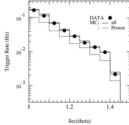
**Fig. 3:** Zenith angle dependence of the trigger rate under any four fold coincidence in the detectors. Each of any four detectors records a signal more than 1.25 particles. Simulation results are compared with the data. Solid and dashed lines show all primary particles and primary protons, respectively.
