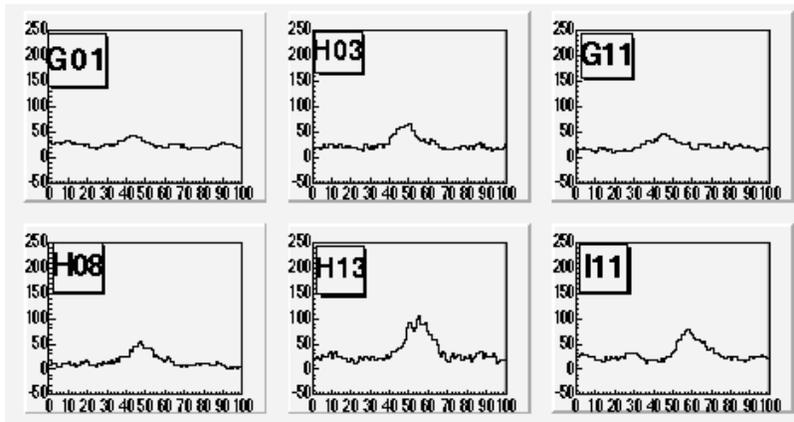
Figure 2: Typical view of a Cherenkov event in several 930 MHz Flash ADC's. Analog and logic delays compensate for the path length differences between the heliostats, so that the signal is centered in each Flash ADC's window. Each window is 100-bin wide, with a bin size equal to inverse Flash ADC's frequency. Signal amplitude is in digital counts (with 2 dc's corresponding to 1 photoelectron)
