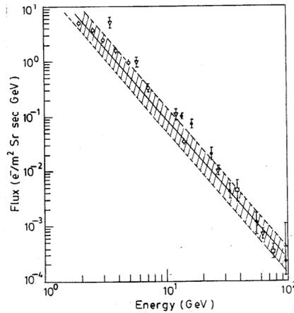
Fig.1. Derived energy spectra of secondary electrons at atmospheric depths 3.8-7.4 g-cm<sup>-2</sup> initiated by p-air collision as described in the text. Broken curves represent the energy spectra at atmospheric depths 3.8 and 7.4 g-cm<sup>-2</sup> and full curve is their mean spectrum. Experimental data: Box Nishimura et al. (1997), bigtriangledown bullet Torri et al. (1996), circ Golden et al. (1994), Basini et al. (1995).
