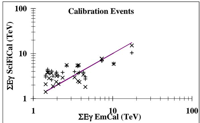
**Fig.4** Comparison of cascade energy determined by EmCal and SciFiCal for 27 events used in calibration. (The cross(x) are the X camera data and the plus(+) the corresponding Y data.)
