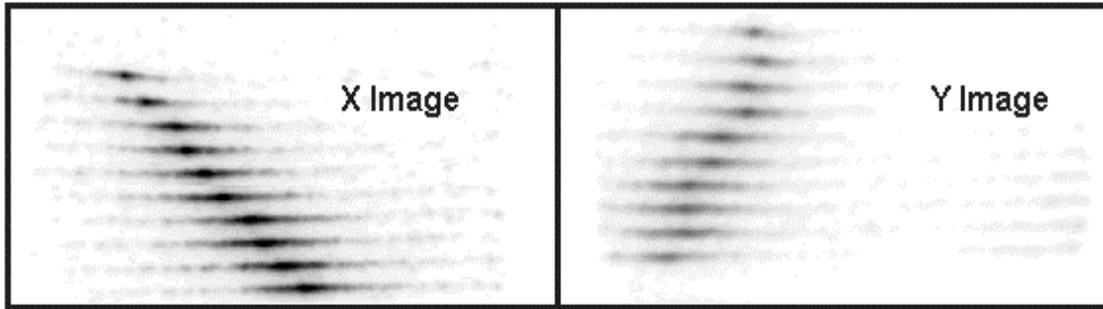
**Fig. 2** Raw images of a cascade in SciFiCal (reverse video). The width of each image corresponds to a continuous segment in the detector 5cm wide. Some blurring of the image was seen which is characteristic of the II-CCDs used.
