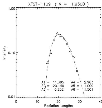
**Fig.3** Transition curve of an event detected in SciFiCal. The event is inclined ( $\tan(\theta)= 1.93$ ).
