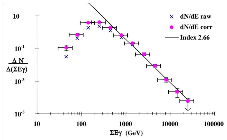
**Fig.5** Differential spectrum measured by SciFiCal. The crosses indicate the measured spectrum and the solid circles have been corrected for the detection efficiency (Christl,1998).
