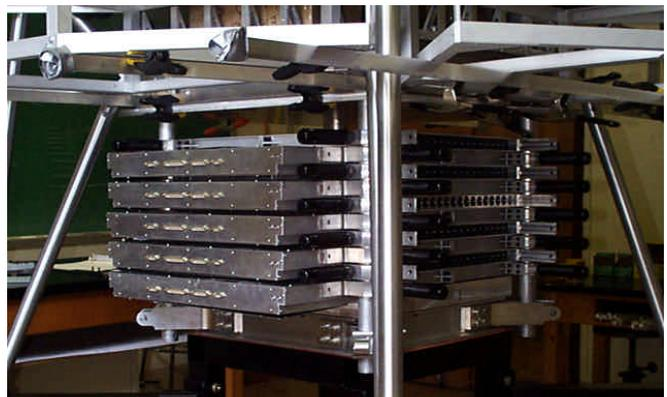
**Figure 3: The calorimeter tray stack**
