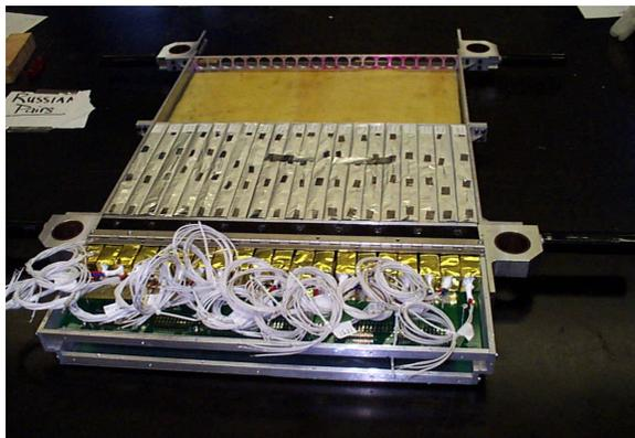
**Figure 2: BGO tray with crystals**
