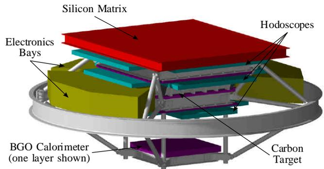
**Figure 1: The ATIC instrument**
