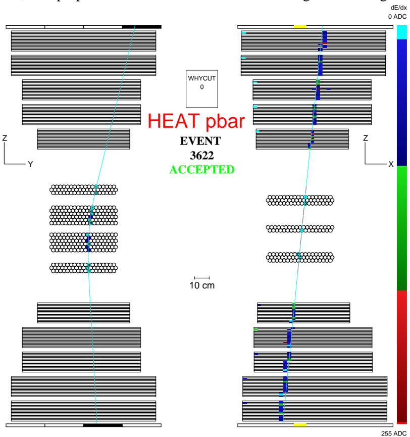
**Figure 3:** Orthogonal views of a sea-level muon passing through the HEAT-pbar instrument with the 1T (central field) magnet on.
