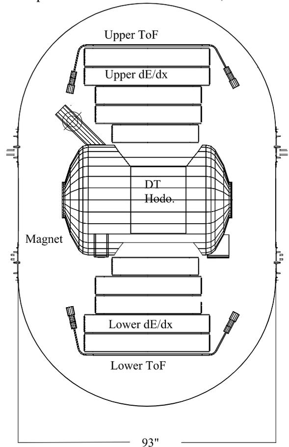
**Figure 2:** Cross-section drawing of the HEAT magnet spectrometer showing the placement of the drift-tube hodoscope in the magnet dewar.
