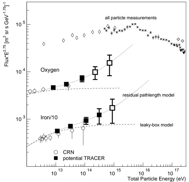
Figure 3: Simulated data for oxygen and iron, indicating the statistical quality of data from TRACER for a 12 day flight.
