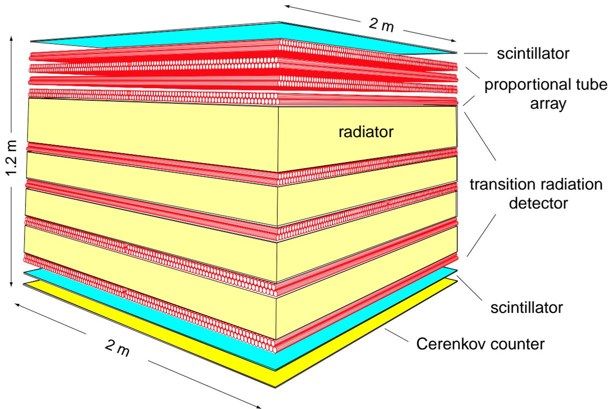
Figure 1: Schematic view of the TRACER instrument.
