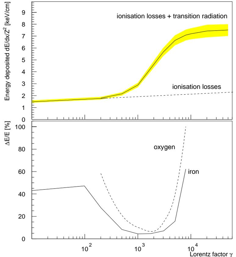
Figure 2: Typical response of a tracer-type TRD to oxygen (upper graph). The dashed line represents the ionization signal without transition radiation that would be measured in the PTA. The expected energy resolution for oxygen and iron nuclei is shown in the lower graph.
