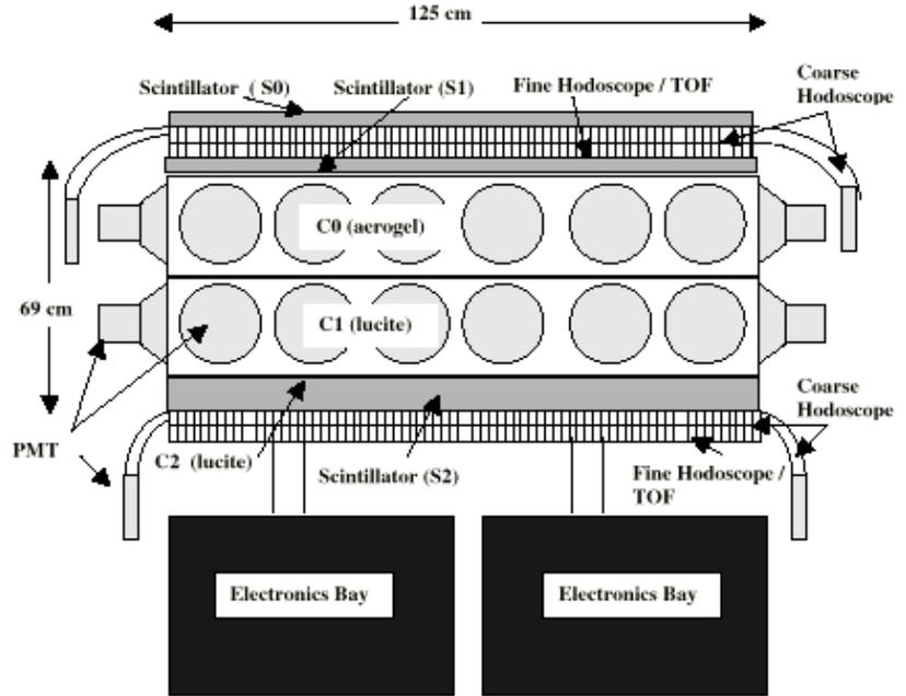
**Figure 1:** Cross-section of the TIGER instrument
