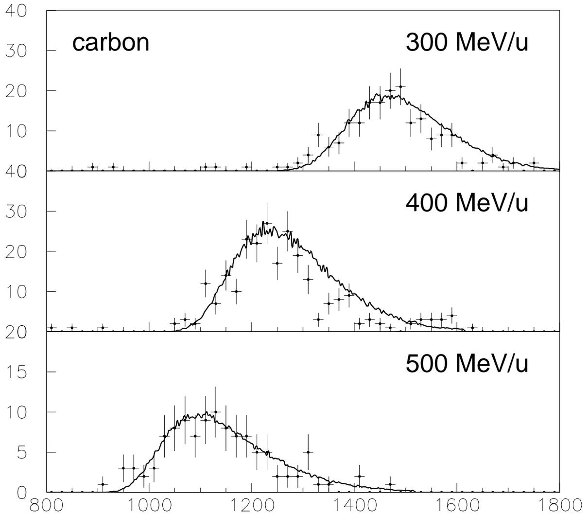
$\beta = 0.654, 0.715$  and  $0.759$ . At these energies,  $dE/dX$  decreases as  $\beta$  increases. Fig. 1 shows typical amplitude distributions for carbon ions measured in the same strip.
