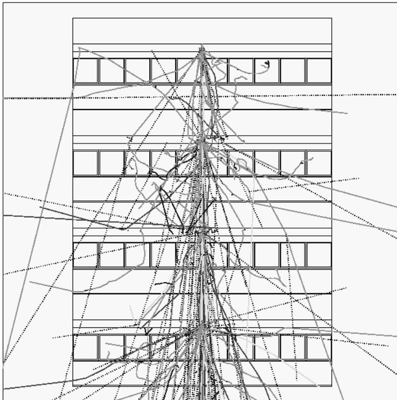
**Figure 1:** A concept for a direct electron pair detector consisting of thin Pb target foils (300  $\mu\text{m}$ ) interleaved with  $x,y$  planes of 1.0 mm square plastic scintillating optical fibers and low mass density spacers to influence the spatial dispersion of the tracks.
