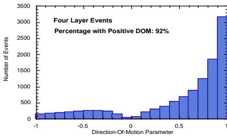
Figure 4: The distribution of the Direction-of-Motion (DOM) parameter for  $^{90}\text{Sr}$  electrons. Positive DOM indicate the correct assignment of the direction of motion.
