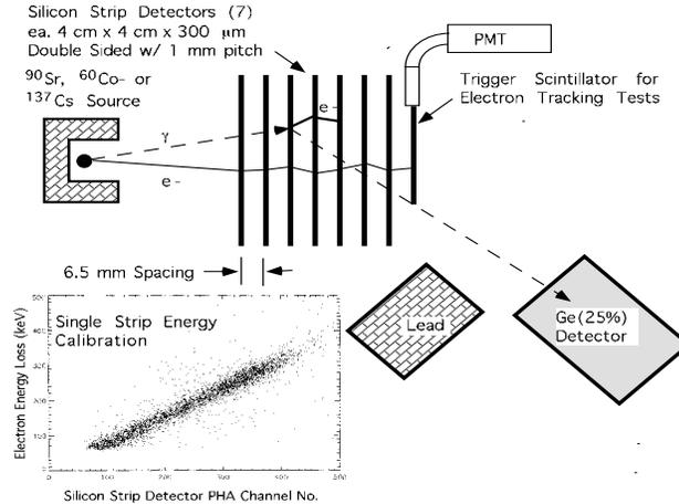
Figure 2: The laboratory setup used for the silicon germanium double scatter experiment.
