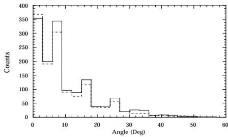
Figure 3: Measured and simulated (dashed line) electron projected scatter angles at 2 MeV.
