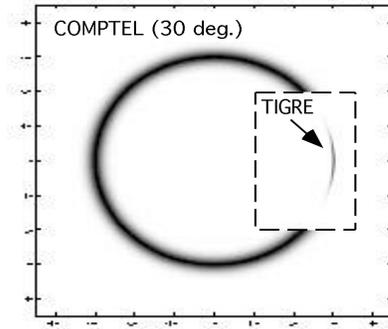
Figure 6: A comparison of TIGRE and COMPTEL PSF showing the great improvement in the incident photon directionality made possible by tracking the recoil electrons.
