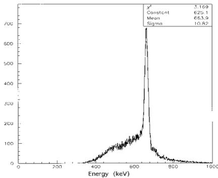
Figure 5: Spectrum of  $^{137}\text{Cs}$  from the Si-Ge double scatter experiment.
