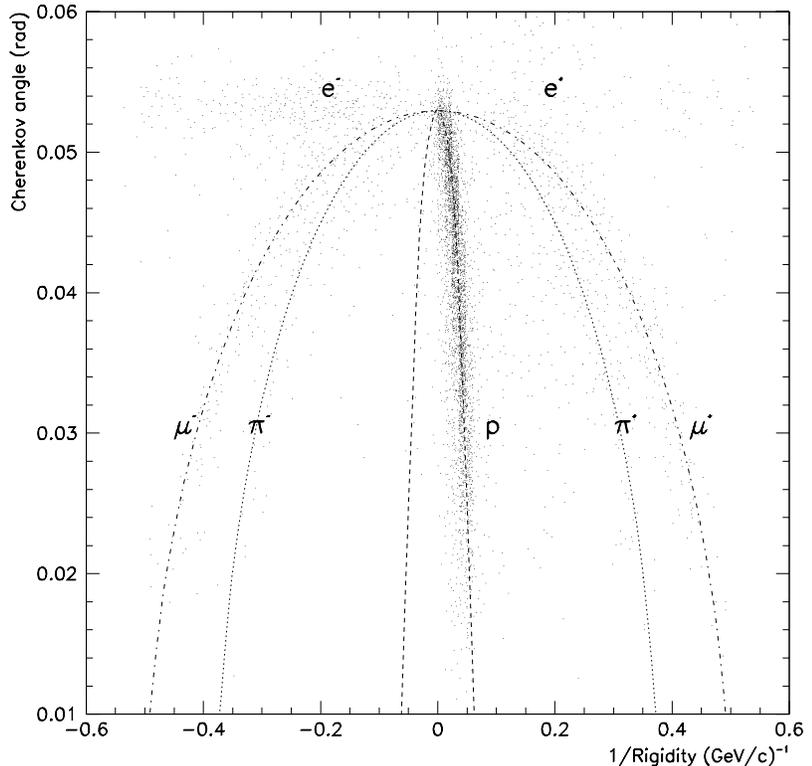
**Figure 2:** The measured Cherenkov angle distribution versus deflection for about 9000 events.
