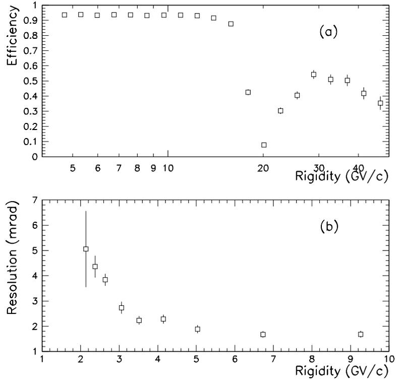
**Figure 3:** (a)The proton selection efficiency for the RICH. (b)The Cherenkov angle resolution for muons as a function of rigidity.
