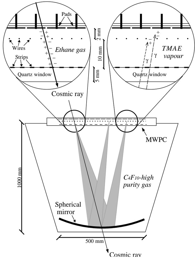
**Figure 1:** Schematic view of the CAPRICE98 RICH detector. At the top are two expanded views of the MWPC. Cherenkov light is emitted in the  $C_4F_{10}$  gas along to the particle track, indicated by the shaded area, and is reflected by a spherical mirror back up onto the photosensitive MWPC.
