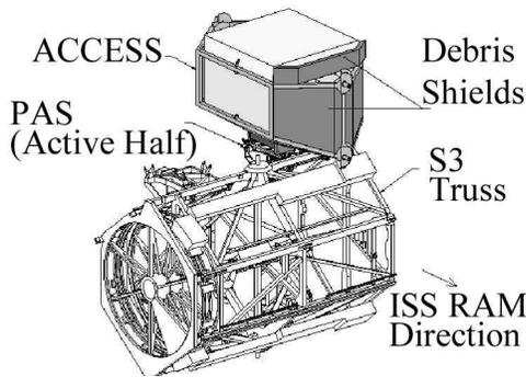
Fig. 5. ACCESS as it Might be Deployed.
