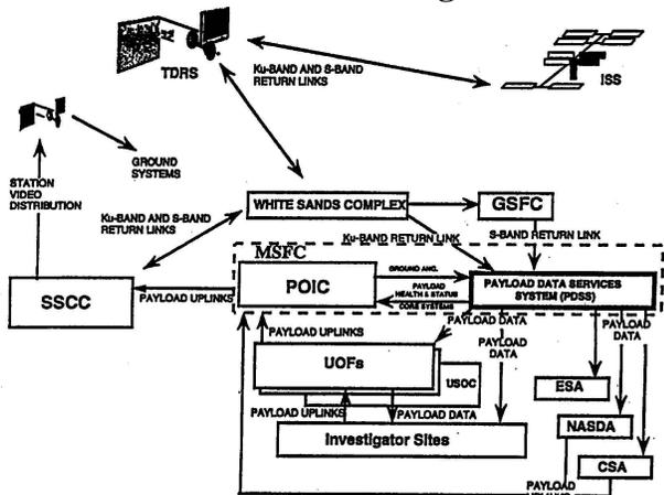
Fig.6. End-to-end ISS Payload Data Flow
