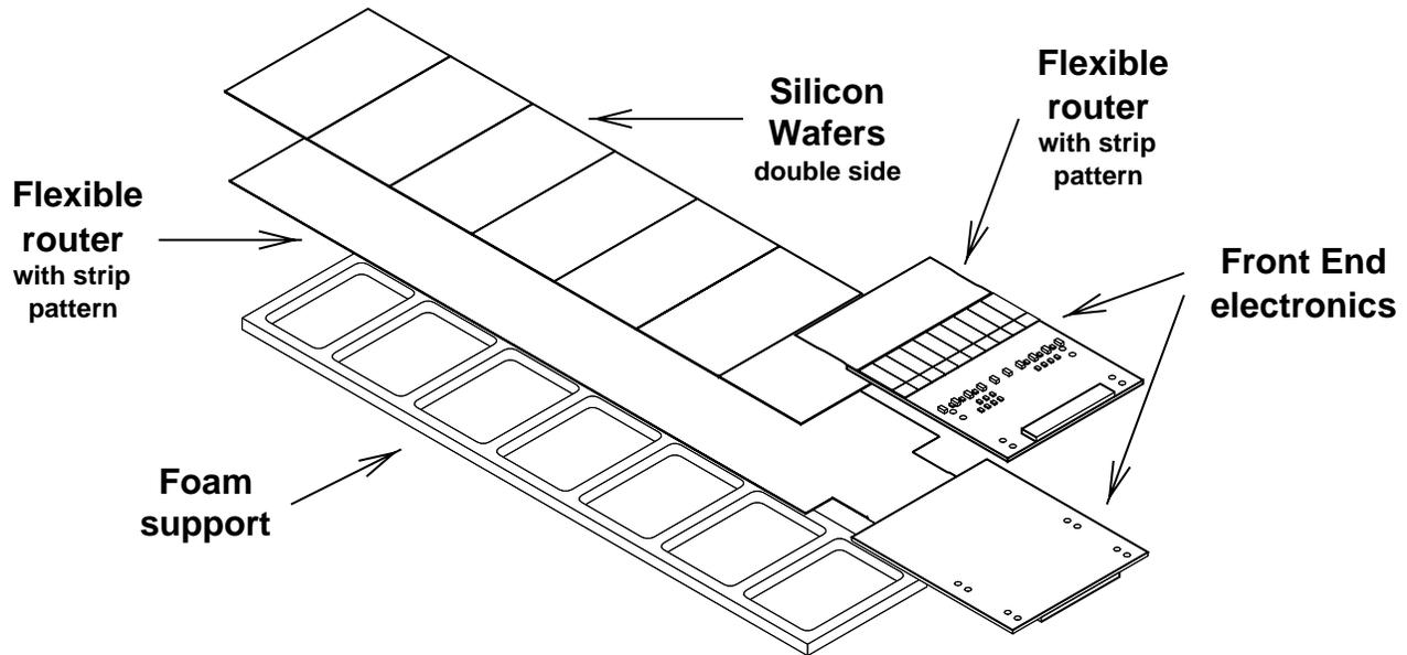
Figure 2: Exploded view of an AMS ladder
