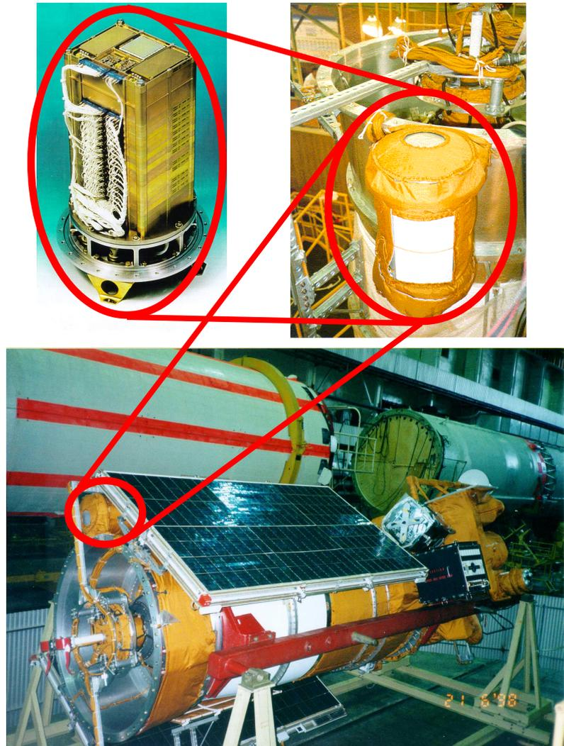
**Figure 1.** NINA apparatus. Top left - The Silicon detector tower without cover. Top right - the detector with cover (note the round acceptance window) being assembled on Resurs. Bottom - the telescope before launch. On the back it is possible to see the Zenit rocket . rocket.
