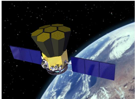
Figure 1: The AXGAM telescope in space showing the seven modules forming a SMEX size instrument.
