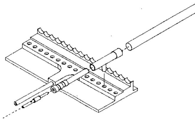
Figure 3: Exploded view of a straw connection to the gas manifold and HV connector.
