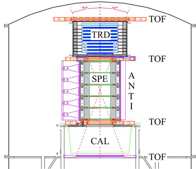
Figure 1: A section of the PAMELA instrument
