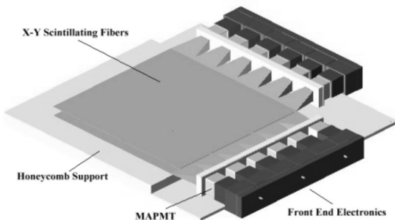
Figure 2 – Closeup of Detector Module Corner
