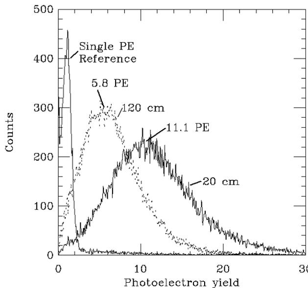
Figure 3 – Light output of 0.75mm mirrored fiber
