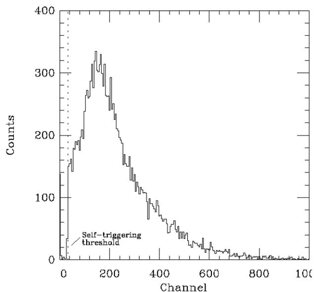
Figure 4 – Typical self-triggered MAPMT anode signal for single photoelectron events
