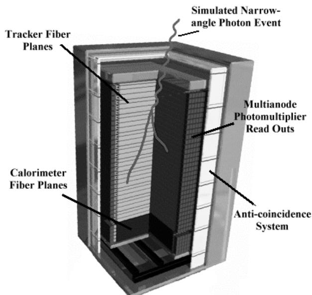
Figure 1 – FiberGLAST Instrument
