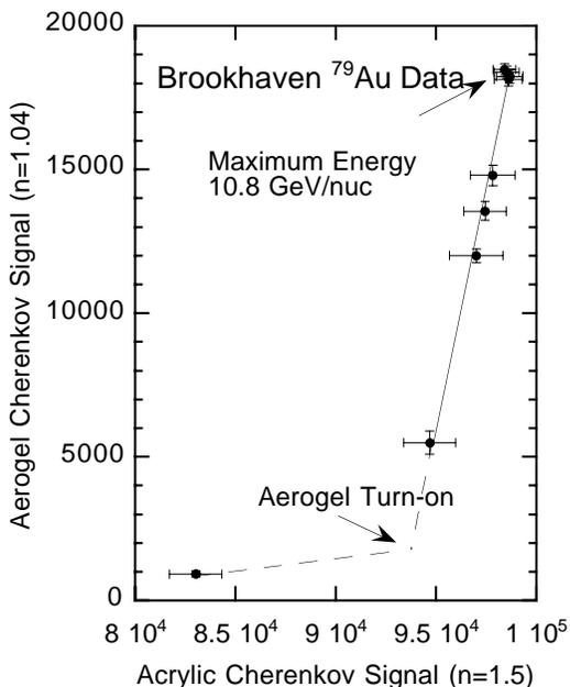
Fig. 5--Aerogel vs. Acrylic Cherenkov Signals
