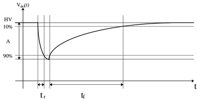
**Figure 3:** Typical semiconductor detector pulse generated by an energetic particle
