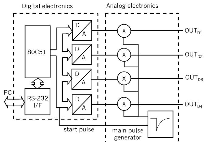
**Figure 2:** MPG block diagram. Enclosed in dashed boxes we can see the analog and the digital modules.
