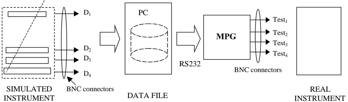
**Figure 1:** Schema of the calibration test using MPG.
