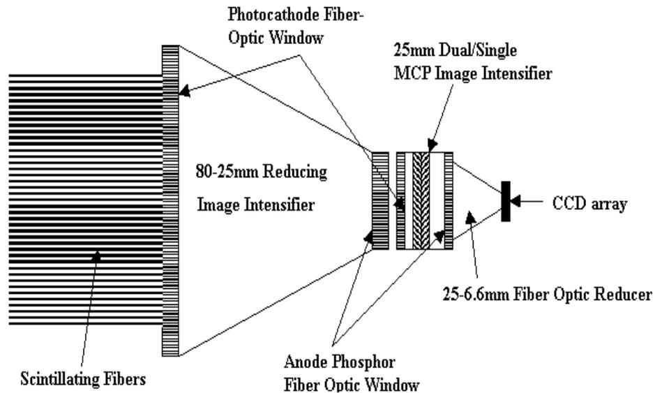
**Figure 2** ICA image intensified CCD read-out system.
