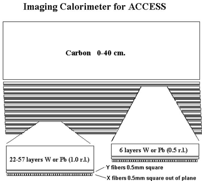
**Figure 1** Schematic of the ICA configuration
