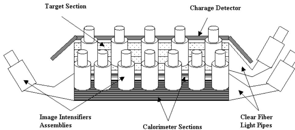
**Figure 3** Schematic of the ICA instrument and IICCD read-out.
