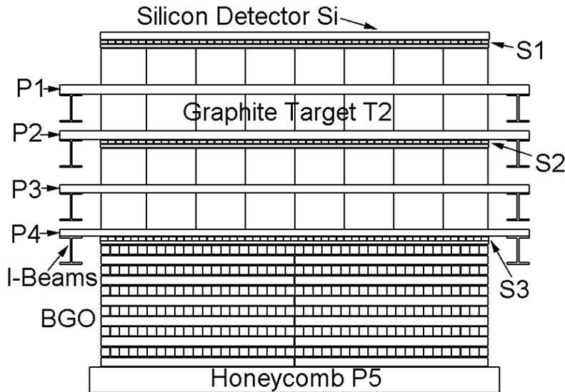
**Figure 1:** Configuration of the ACCESS baseline calorimeter
