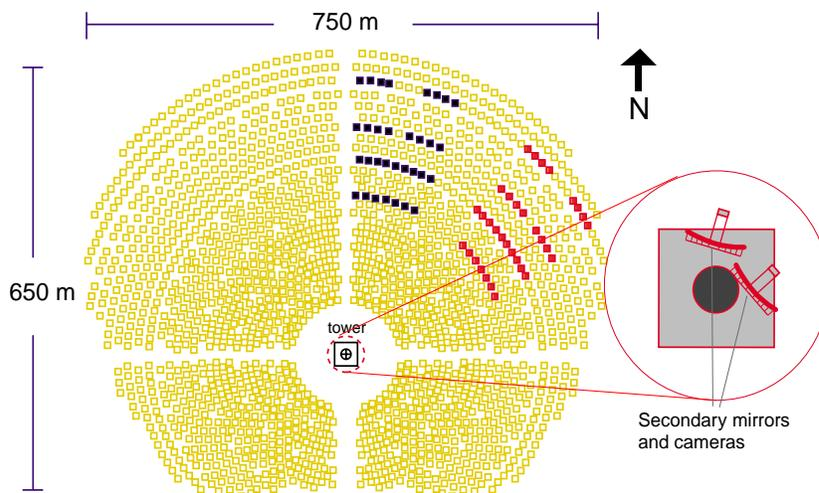
**Figure 2:** Schematic aerial view of the Solar Two heliostat field and tower. The 32 heliostats that will be viewed by the first secondary are the filled, blue squares in the upper left of the northeast quadrant. The filled, red squares on the east side of the northeast quadrant are the 32 heliostats to be viewed by the second secondary. We plan to build a third secondary to view an additional 32 heliostats closer to the central tower.
