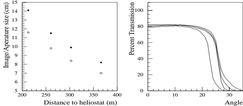
**Figure 4:** On the left, the maximum heliostat image size in the focal plane (filled circles) and the entrance aperture diameter (open circles) are plotted as a function of the distance from the heliostat to the secondary mirror. On the right, the transmission of the cones as a function of angle is plotted.
