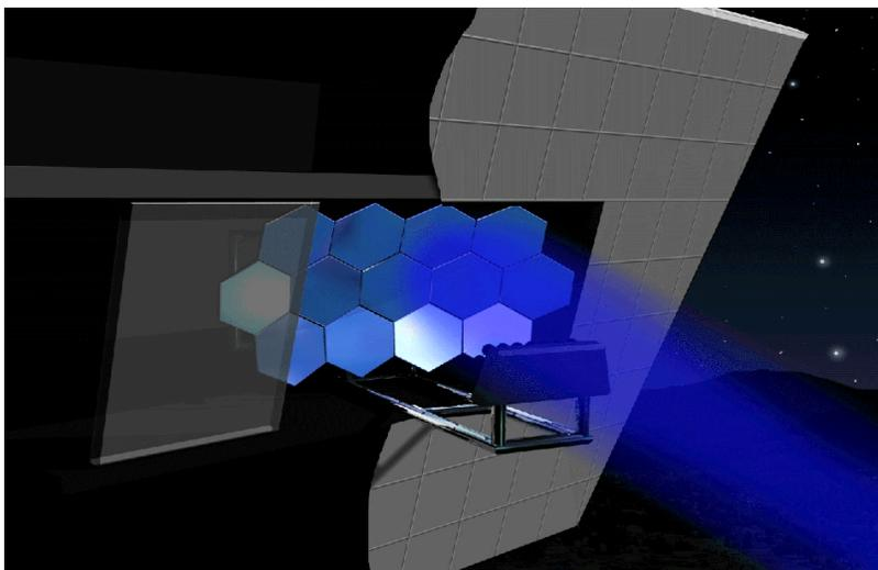
**Figure 3:** Illustration of the secondary mirror and camera mounted in the central tower at the Solar Two Power Plant. The secondary has a 6 meter radius of curvature is composed of 13 1 meter hexagonal facets, each with a 6 meter radius of curvature.
