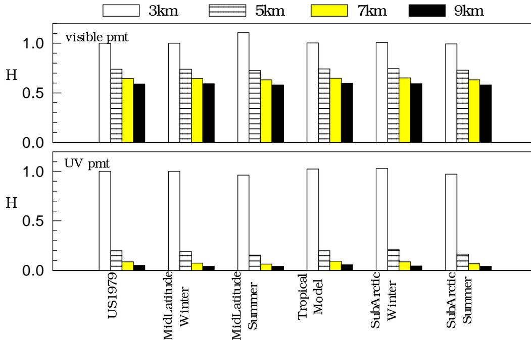
**Fig. 3.** Seasonal dependence of the response of atmospheric Cherenkov telescope with visible and UV cameras.
