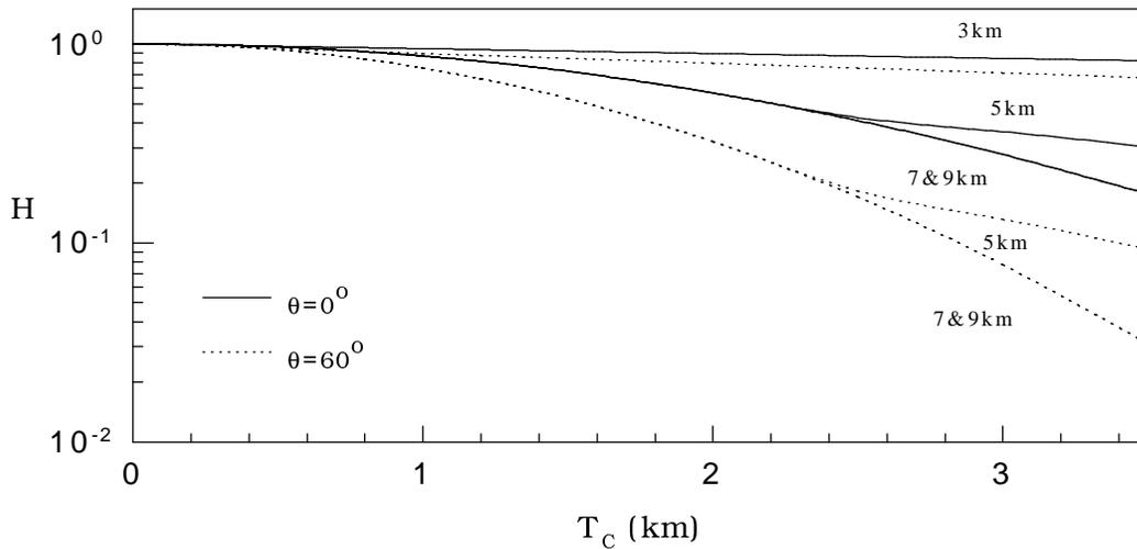
**Fig. 2.** Variation of the relative response function of the visible or UV photomultipliers with the cirrus cloud thickness for light generated at 3, 5, 7, and 9 km and detected at 2.3 km. The zenith angles are 0 and 60° and the cloud base is at 2.6 km.
