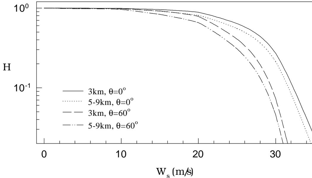
**Fig. 1.** Variation of the relative response function of the visible photomultipliers with the wind speed for light generated at 3, 5, 7, and 9 km and detected at 2.3 km. The zenith angles are 0 and 60°.
