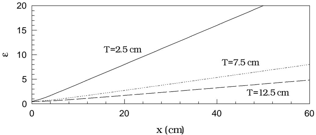
**Fig. 1.** Results of Monte Carlo simulation of the variation of the parameter  $\epsilon$  of the direct light component with the distance  $x$  for different scintillator thickness.
