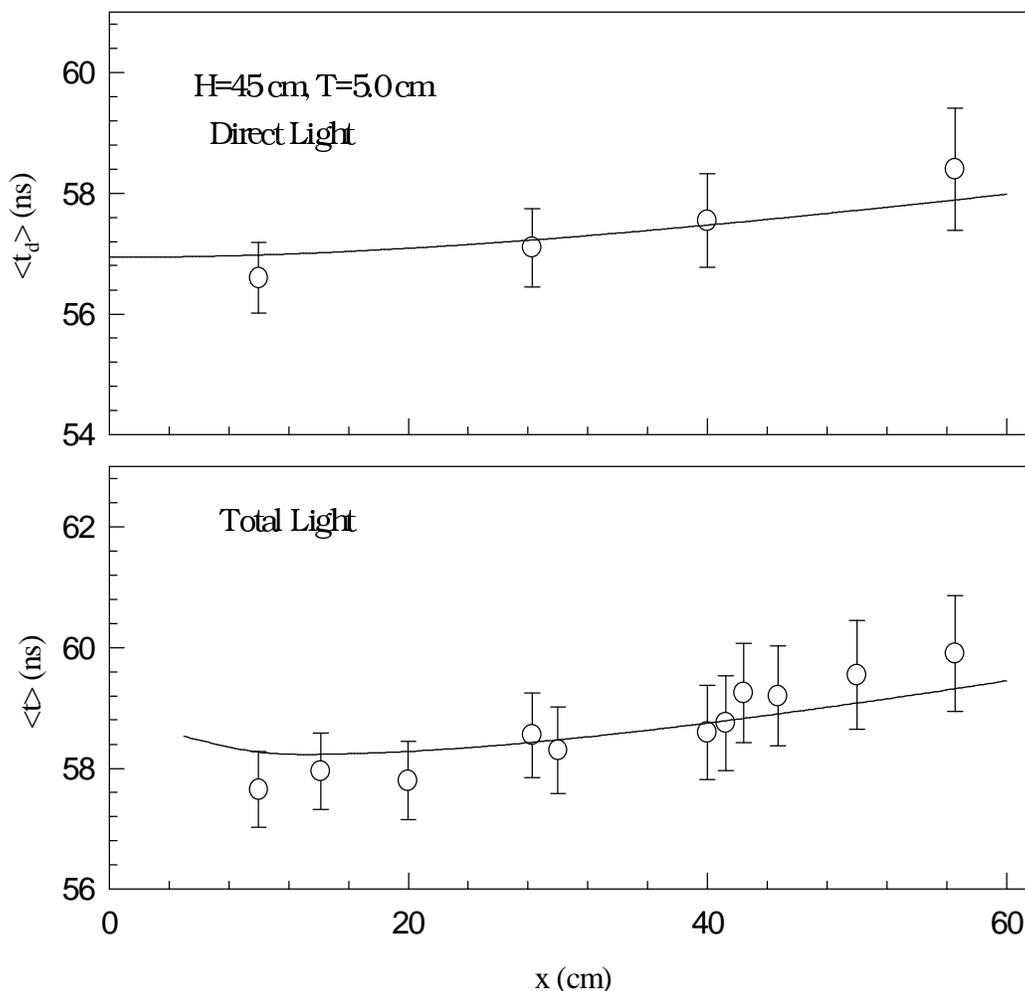
**Fig. 2.** The measured average time as a function of the distance  $x$  for the direct light component and the total light using 3.5 GeV electrons. The solid lines are the results of the calculations of the present model.
