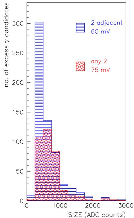
Figure 3: SIZE distribution of  $\gamma$ -ray candidate events after background subtraction (see section 2.2) for the 2-fold PST and the 2-fold coincidence (hatched area) triggers recorded at 60 mV and 75 mV discriminator thresholds respectively.
