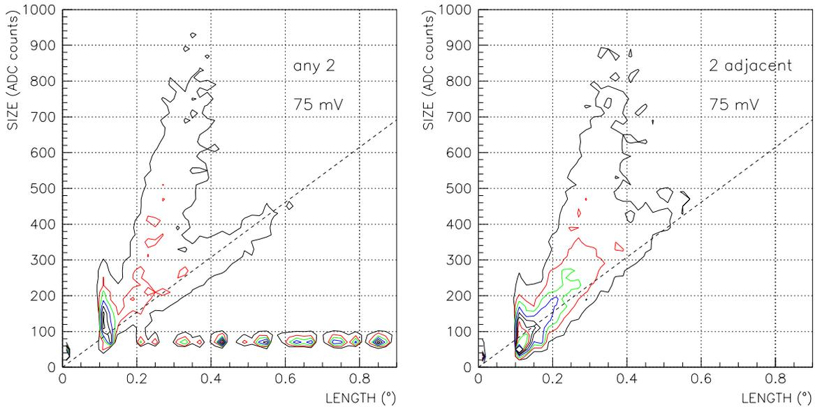
Figure 2: Comparison of calibrated image SIZE as a function of the Hillas parameter LENGTH for data recorded at a discriminator threshold of 75 mV with the 2-fold coincidence trigger (left) and the 2-fold PST (right). Contours indicate 30 to 300 events in 30 event steps.
