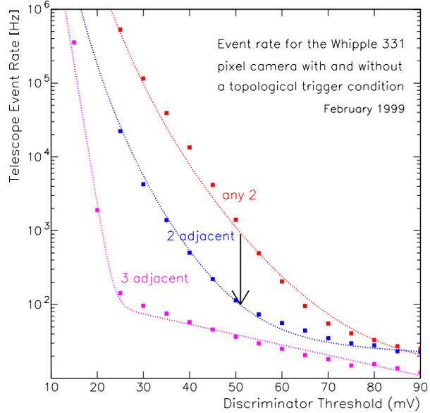
Figure 1: Whipple 10m telescope trigger rate as a function of discriminator threshold (February 1999).
