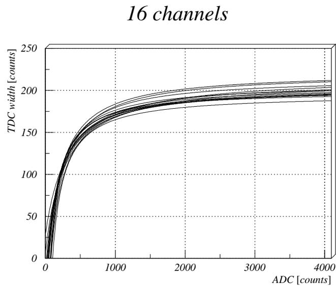
**Figure 3:** An example of the pulse height vs. pulse width (or time over threshold) curve. Sixteen curves from 16 PMTs assembled in a module (Figure 1) are shown. These are measured in a laboratory with the same electronics and cables using an LED light source.
