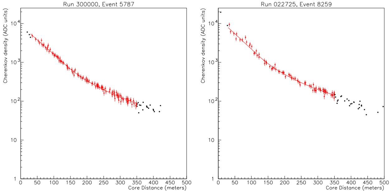
Figure 1: Sample Cherenkov lateral distributions. *Left*: 1 PeV proton simulation. *Right*: An actual shower.
