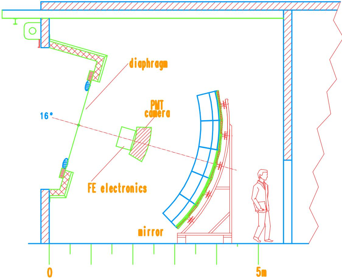
Figure 1: Diagram of Auger telescope design.
